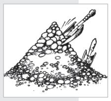
Fig. 2: Sampling from a heap of sand
