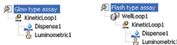
Figure 4. SkanIt software measurement protocol steps for glow and flash type reactions. The protocol on the left can be used for the slower kinetics of glow type ATP reaction and the protocol on the right is optimal for the fast flash type kinetics, where the interval time of kinetic readings must be short.
