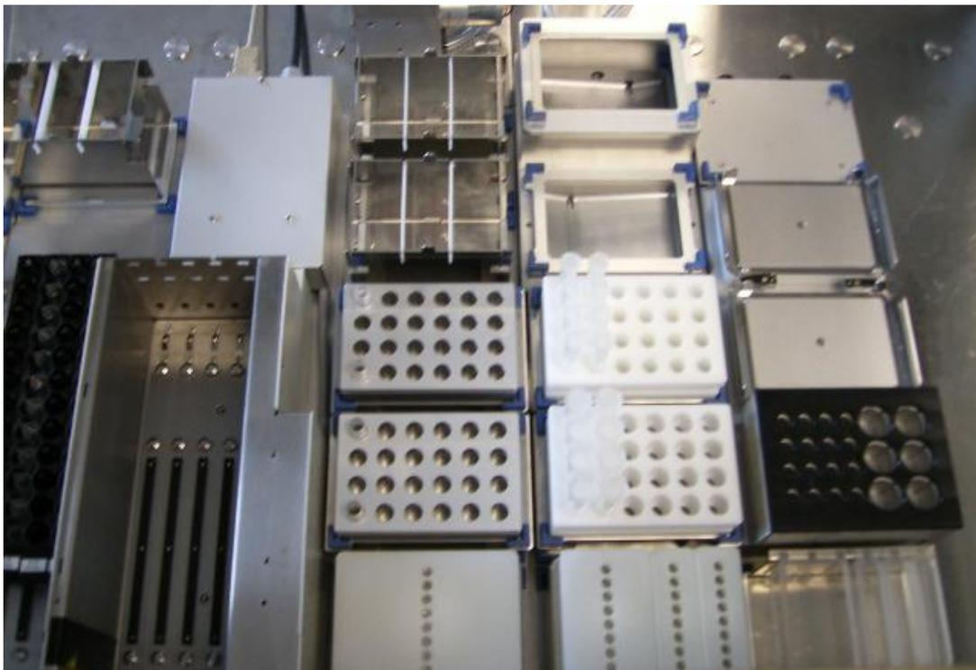
*Fig 3: CyBI®-RoboSponse deck layout for peptide mapping*
