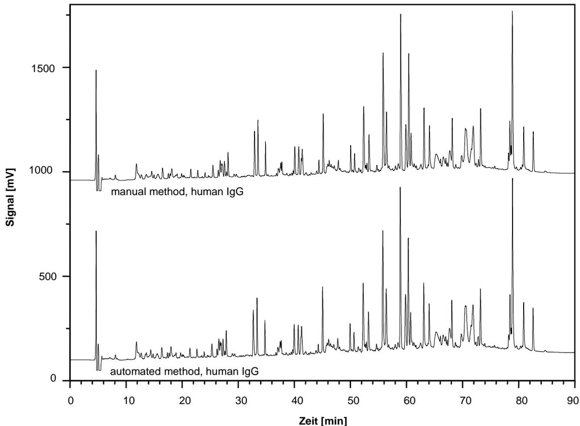
Fig 4: Comparison of manual and automated processing of the same protein analyzed with an Agilent HPLC system.
