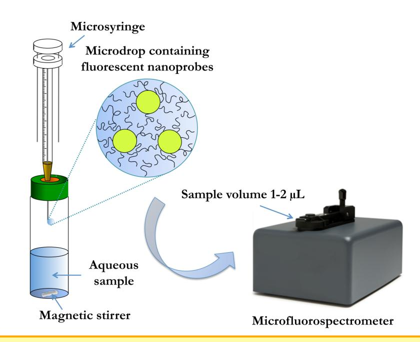
CdSe QDs functionalized with hexadecylamine as luminescent probe for the selective and sensitive detection of selenium
