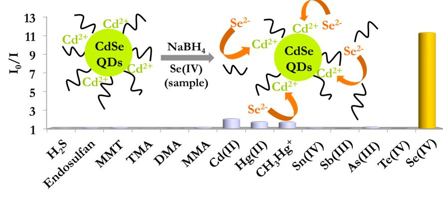
Luminescence quenching occurs as a result of the binding between exogenous selenide trapped into the organic drop and Cd<sup>2+</sup> contained in the QDs structure, which may cause the loss of stabilizing agent and, in turn, the luminescence quenching.
