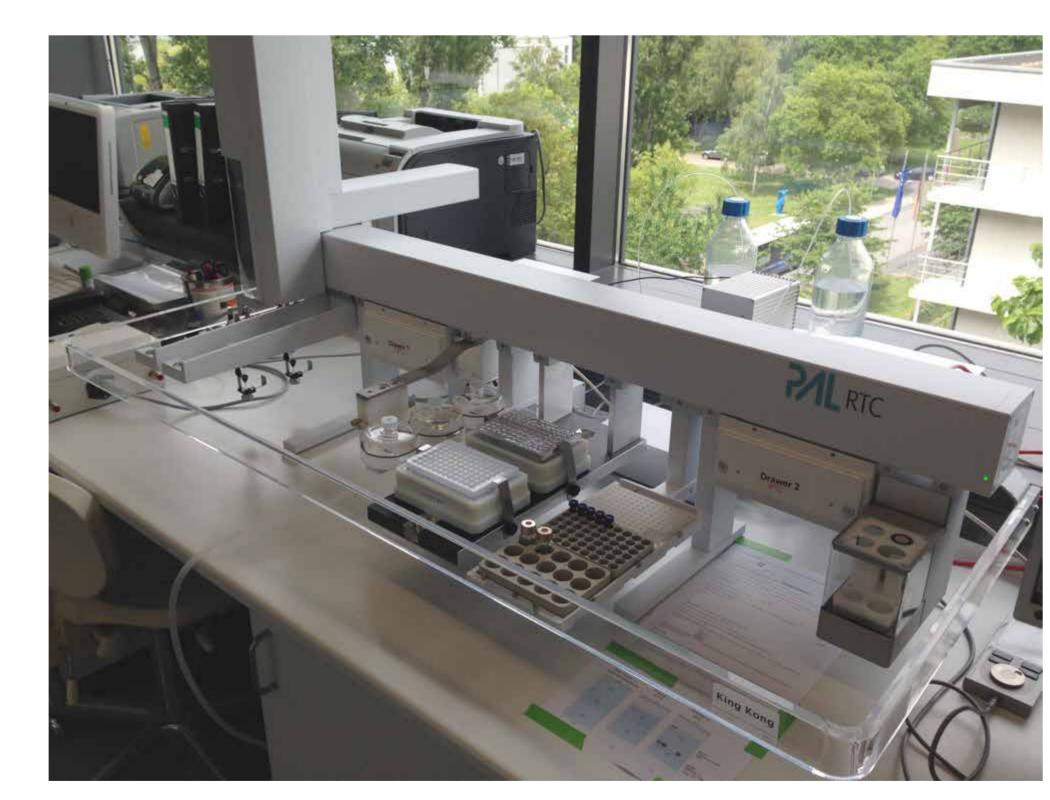
A representation of an RTC-PAL setup. Each module is variable and thus the robotic setup can be extended by introducing new tools.
