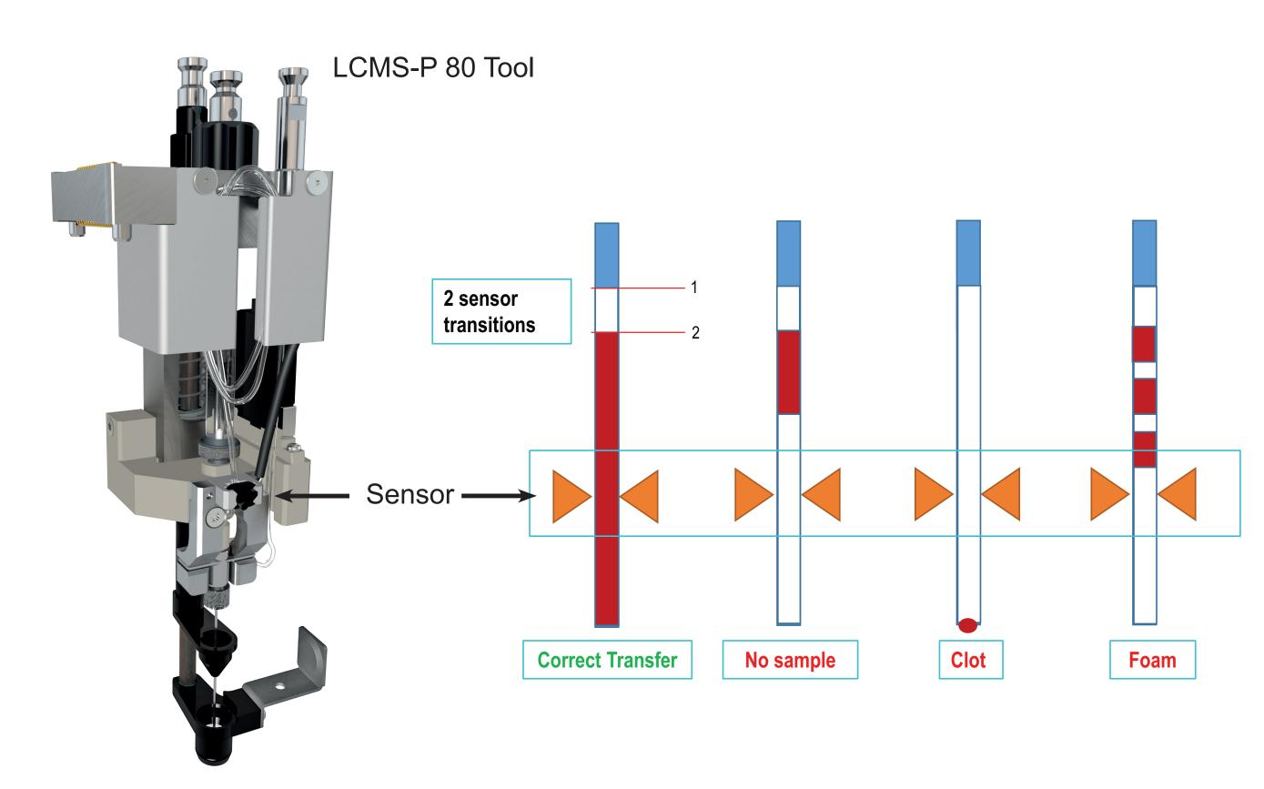
The optical sensor positioned on the sample loop (orange triangles in the sketch above) of the tool moitores the aspiration of sample, air gap or bubbles. Different sampling situations (injection with air gaps, clogging, bubbles) generate distinct patterns of the sensor signal triggering defined actions of the system.
