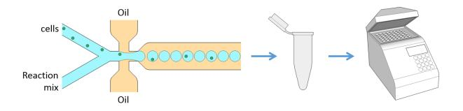
**Figure 1**. In a typical experiment, cells are combined with a reaction mix, such as an RT-PCR mix, and encapsulated in droplets in oil. The resulting micro-emulsion is collected, typically in a chilled PCR tube, and transferred to a PCR machine for RT-PCR.
