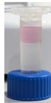
Eppendorf tube with 200 µL of overlay fluid on top of Pico-Surf2™ oil
