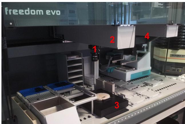
Figure 1 Freedom EVO with Pickolo module consisting of a camera (1), mounted on the LiHa (2) and the backlight carrier (3). Petri dishes are transported by the RoMa (4).
