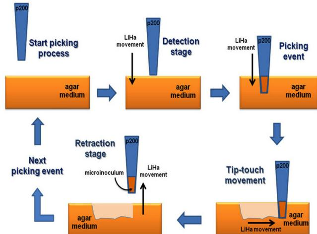
Figure 4 Graphical overview of the unique procedure for picking fungi from hard agar.
