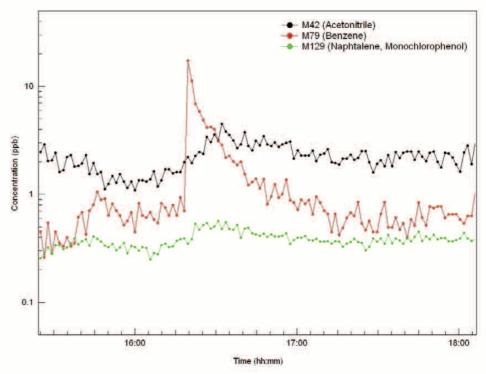
Fig. 2: Online exhaust gas measurement of a waste incineration process.
