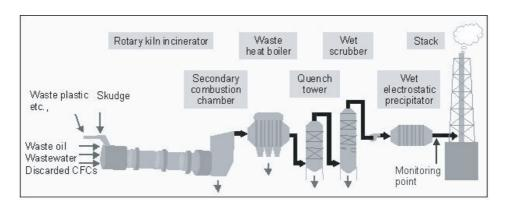
Fig. 1: Schematic drawing of experimental set up.
