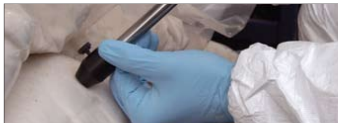
Figure 2. The nosepiece eliminates stray light and keeps the sample at the optimum focus distance from the probe.
