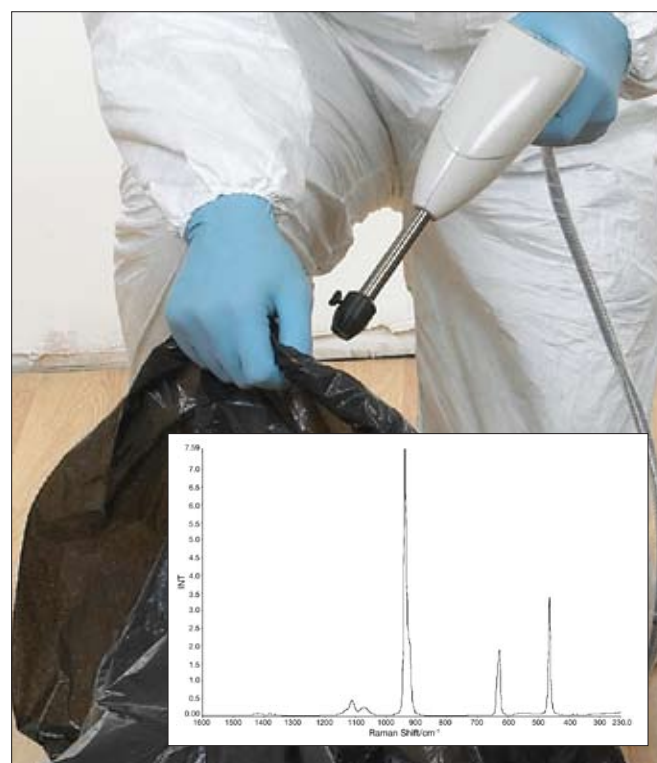
Figure 6. Raman spectra can be obtained through a variety of containers including black plastic bags. The spectrum is of ammonium perchlorate explosive through black plastic bag.
