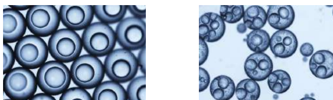
Left: Double emulsions made up of an aqueous core (w), an organic shell (o), and an aqueous continuous fluid (w). Right: Oil droplets with multiple water droplets within. Typical droplet sizes range between 50 \mu m and 150 \mu m.
