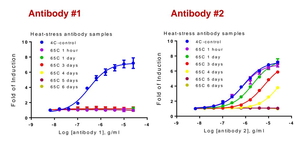
Detecting loss of reporter response to PD-1 or PD-L1 blocking antibody after heat-treatment: Anti-PD-1/PD-L1 blocking antibody #1 and #2 were heat stressed at either 42°C or 65°C for indicated times before application to thaw-and-use cells in the PD-1/PD-L1 Blockade Bioassay. Loss of reporter response to heat-stressed anti-PD-1/PD-L1 blocking antibody after heattreatment was detected.
