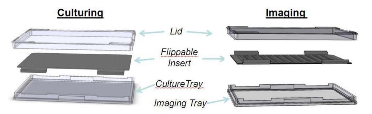
Figure 1: Schematic of the µALI Plate. The µALI Plate consists of a single 96-well flippable insert which allows liquid handling access and contains both the basal and apical sides of the device. The insert can be placed in a culturing tray for cell culture or removed and placed in an imaging tray for high content imaging.
