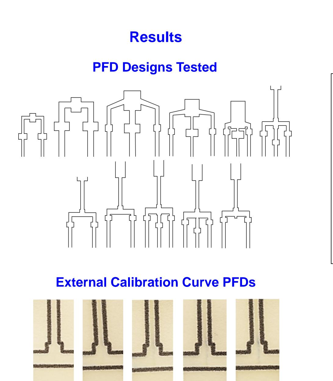
Water drives the phosphate-containing sample and the combined reagent vertically through the channels until mixing is completed producing a blue color (Antimony-Phosphomolybdenum Blue) in the presence of phosphate
