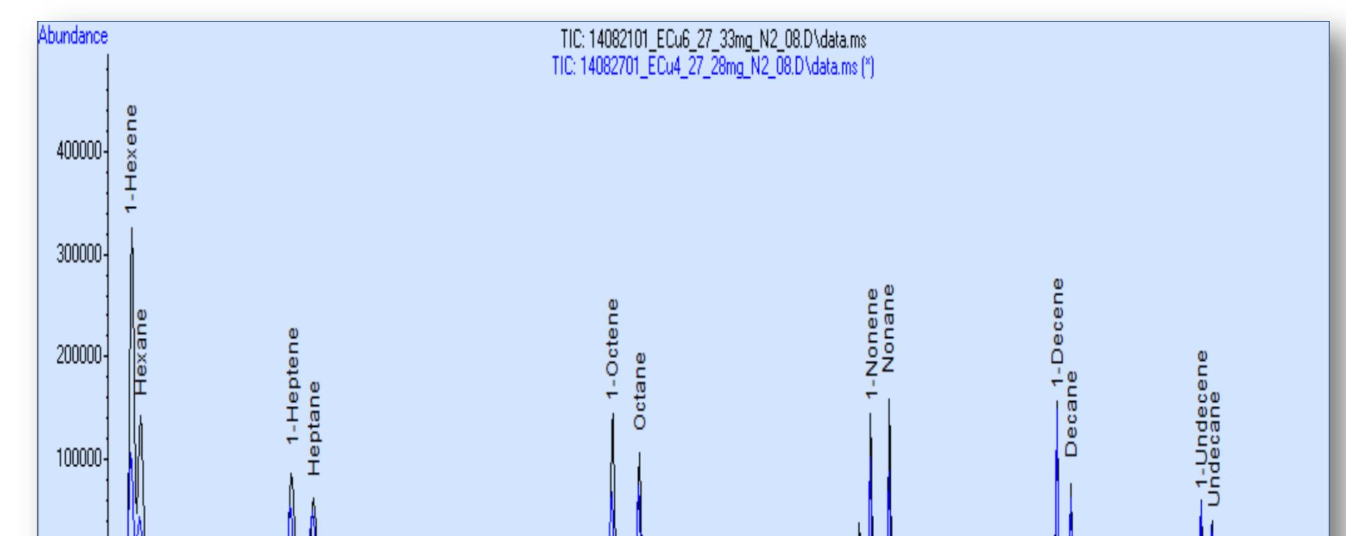
Hexane and hexene signals increase with the quantity of octene in the sample
