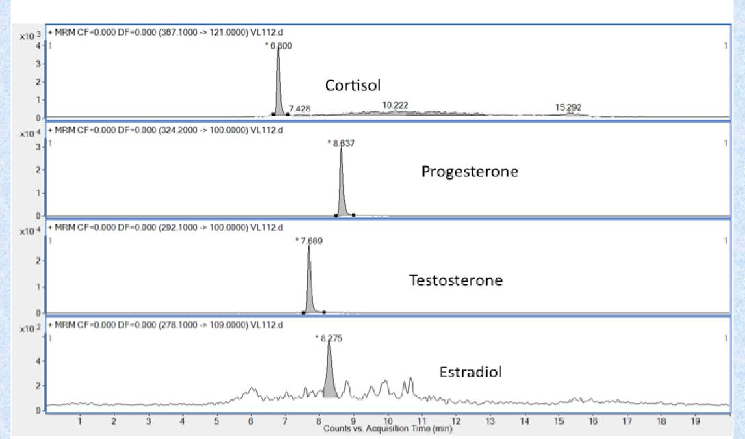
Figure 1: Sample extracts were submitted to the Purdue University Proteomics Facility and analyzed on a Agilent 6460 Triple Quadrupole mass spectrometer coupled with the Agilent 1200 Rapid Resolution high-performance liquid chromatography (HPLC) to validate the identity of the measured hormones (e.g., Lupica and Turner, 2009). The graph above, shows detectable limits of all steroid hormones.
