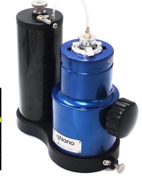
Tuning the pore size, applied pressure and voltage improves the measurement sensitivity and enables a wider range of particles to be analysed.
