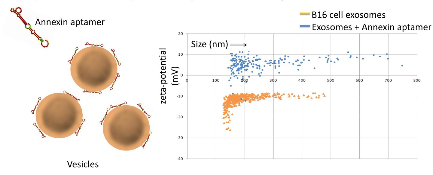
The interaction of aptamers with biological targets on the vesicle surface, e.g. CD63, can provide discriminatory information based on the size and charge profiles of the different populations.
