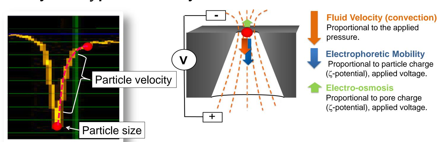
$\zeta$ -potential is calculated from the shape of the resistive pulse signal generated. Changes to the particle surface through, for example, protein or aptamer binding can cause changes in  $\zeta$ -potential. Due to the particle-by-particle measurement, mixtures of vesicles with different surface properties can be measured.
