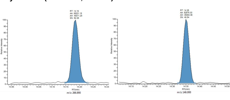
The instrument LOD was assessed by repeatedly (n = 20) injecting the 10 ppb (0.01 mg/kg) calibration standard taking into account the student's-*t* critical values for the corresponding degrees of freedom (99% confidence), the concentration of each native compound, and %RSD. The results of this test show excellent LODs for the pesticides analyzed with values between 1 ppb (200 fg on column) (Boscalid) - 3 ppb (600 fg on column) (Chlorfenapyr) (Figure 4).
