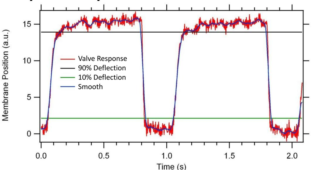
A valve was actuated at 1 Hz and 30% duty cycle. Fall time (valve closure) was 0.019 s and rise time (valve opening) was 0.105 s. No vacuum was used to open the valve, and the fluid backpressure was negligible.
