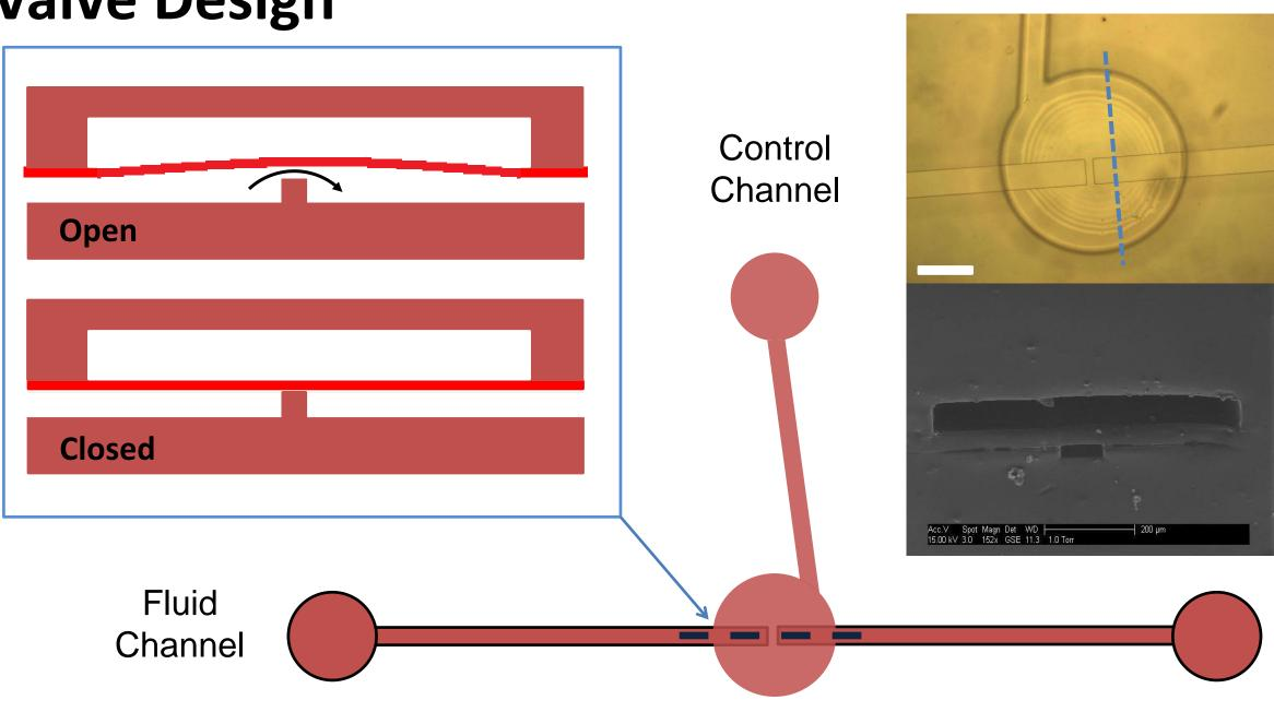
Schematic of a three-layer poly-PEGDA valve. The left inset is a cross-sectional view along the dashed line for an open or closed valve. (Right top) Top-view photomicrograph of a valve. Interference fringes indicate that the membrane is deflected upward (valve open) after the final bonding step. White scale bar is 200 μm. (Right bottom) SEM of a valve cross-section along the dashed line in the photo.
