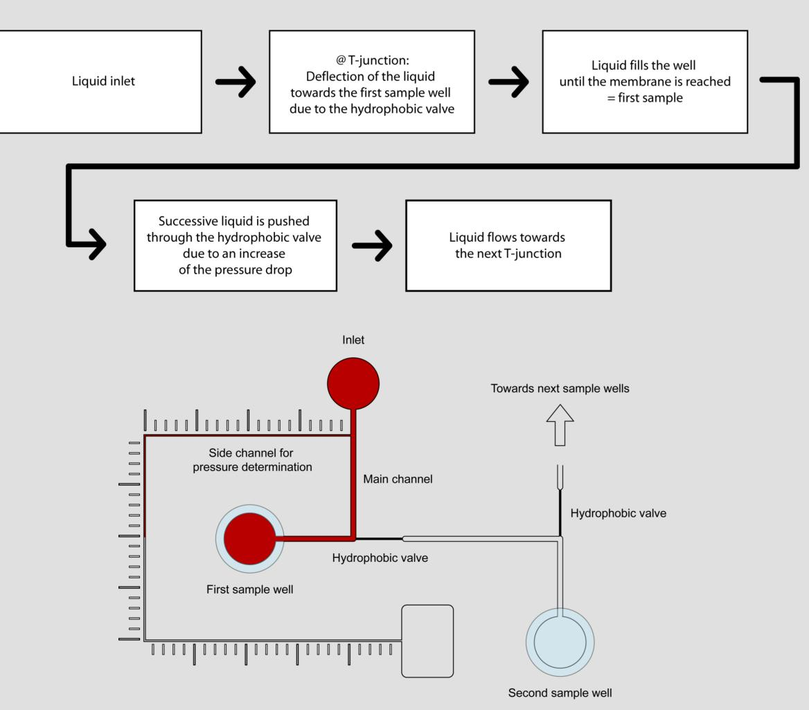
For the determination of the valve burst pressure, we integrated the side channel ( $150\mu m \times 150\mu m$ ) in the milling step. From the amount of liquid, that was pushed inside the channel before and after the valve burst, the bust pressure could be determined. The mean pressure value was 700Pa, which is in the range of the expected theoretical value.
