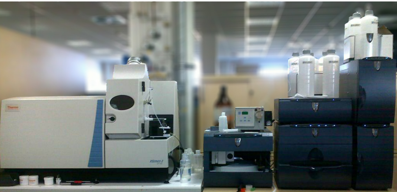
Figure 1. IC-ICP-MS system: Dionex ICS-5000 system coupled to XSERIES 2 ICP-Q-MS system
