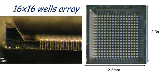
The micro-wells array is a matrix of micro-cavities closed with a thick membrane (2µm) of  $SiO_2/Si_3N_4/SiO_2$  multilayer. The the twofold has membrane advantage of being transparent and strong enough to act as a plug.
