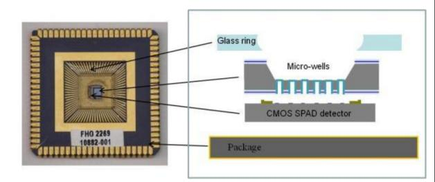
All the biofunctional, fluidic and detection layers will be integrated in a single package
