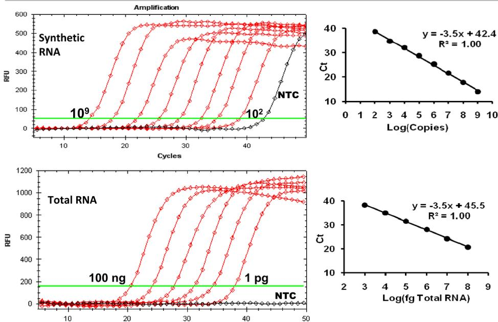
100 copies of miR21 could be detected from synthetic RNA standard or 1 pg of Total RNA.
