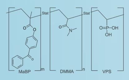
Chemical structure of the copolymer: DMMA: monomer, basis for the polymer chains MABP: photo radicalic cross linker VPA: enhances solubility in water
