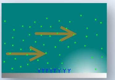
Lateral shifting of the depletion zone via pressure driven flow of analyte solution
