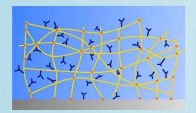
Schematic illustration of a spot containing antibodies immobilized in polymer network
