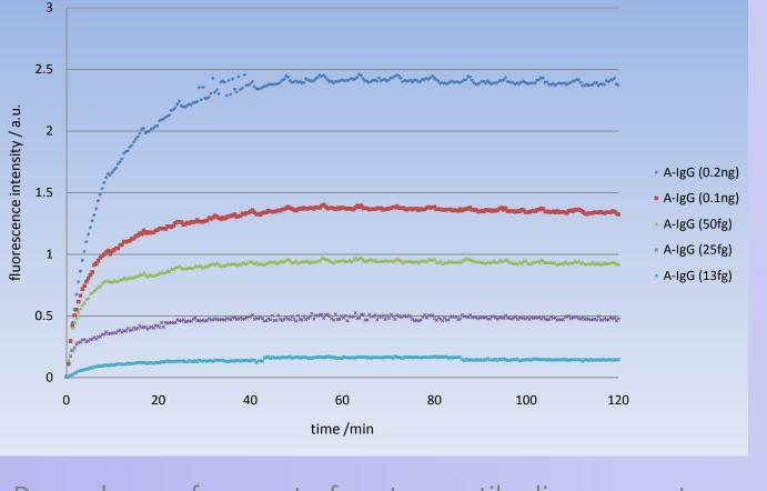
Dependence of amount of capture antibodies per spot on the fluorescence signal. Concentration of Cy5-labeled human IgG in solution: 8 nM
