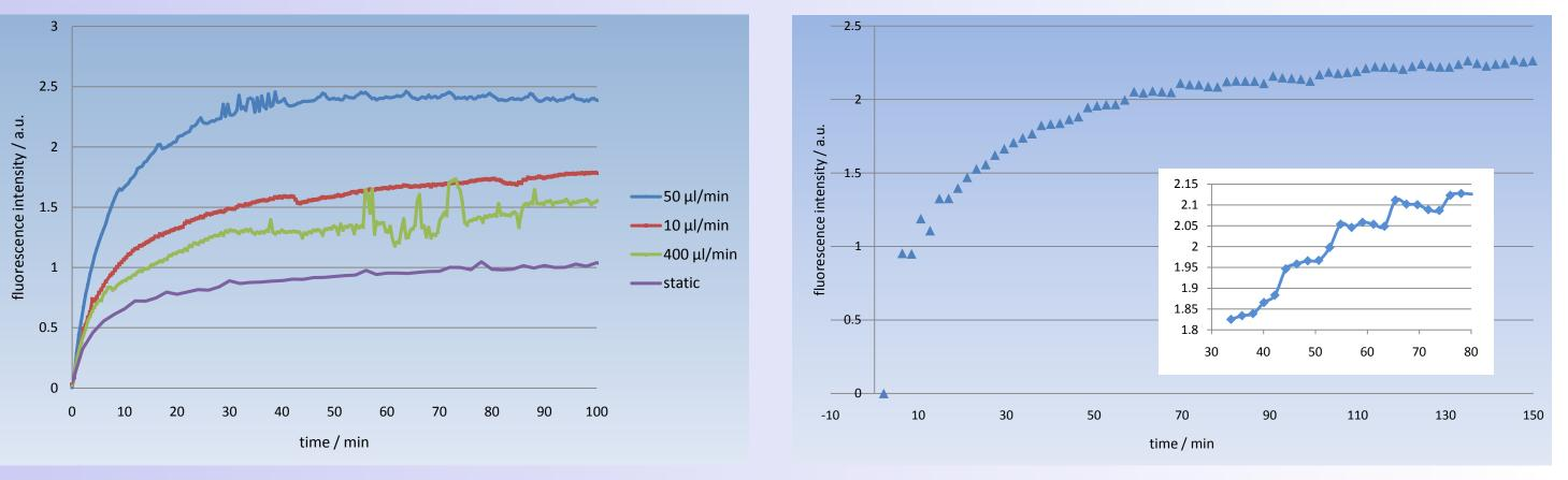
Dependence of the flow rate on the fluorescence signal. Concentration of Cy5-labeled human IgG in solution: 8 nM
