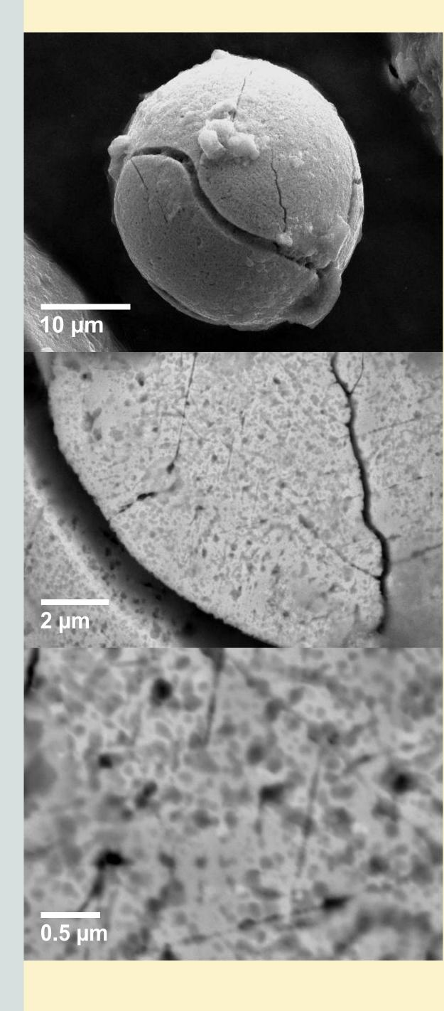
A 28 µm diameter uranium oxide sphere from a wind-blown dirt sample (dirt: 379  $\pm 21$  mg/kg U,  $^{238}$ U/ $^{235}$ U 469 ± 14). Preserved in a sheltered environment.
