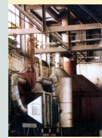
Scrap uranium metal was converted to oxide in a furnace that vented to the atmosphere (left). The plant (below right) was closed by the authorities in 1984 for excessive uranium emissions to the environment, and has now been remediated with the removal of 180,000 tonnes of soil<sup>2</sup>(below left). Uranium contamination is evident in a sediment core from downstream of NLI<sup>3,4</sup>.
