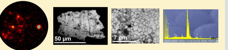
Images from left to right: Autoradiography of density-separated particulate on SEM mount, SEM image of particle highlighted by autoradiography, close-up showing agglomerated texture, EDX spectra from spot analysis.
