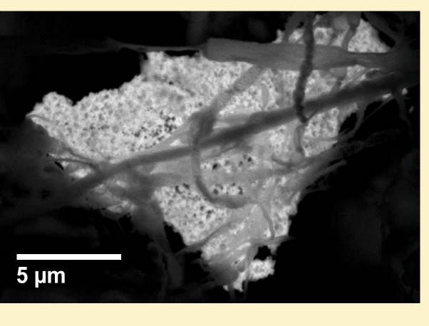
A uranium bearing particle adhered to the surface of a wooden fence post. It appears porous and sponge like. This could be from advanced degradation in an exposed environment.
