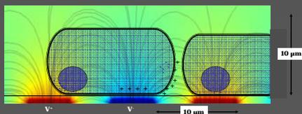
Figure 4: FEMlab simulation of electric potential distribution using the present sensor geometry.
