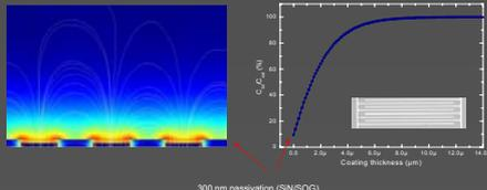
Figure 3: FEMlab simulation of dielectric displacement using the present sensor geometry of 200 fingers with 5 x 5  $\mu\text{m}$  width and gap. Calculation of electric field distribution using conformal mapping technique.
