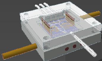
Figure 2: Design drawing of the microchip comprising of a glass bottom and a polymer (PDMS) cover and fixture.
