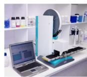
mosquito is a low volume liquid handling instrument combining a low cost disposable tip system with a positive displacement pipette. mosquito is capable of pipetting volumes from 1.2  $\mu$ L down to 50 nL with no washing required.
