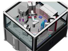
TTP LabTech and Velocity 11 have designed a fully automated high content system incorporating mosquito to perform primary and secondary screens on a compound library. A single system could screen a library of up to 400,000 compounds for hits and then validate those hits in less than 1 week.
