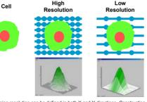
Scanning resolution can be defined in both X and Y directions. Construction of 3D fluorescence intensity profiles permits the calculation of fluorescence and morphological parameters for each object identified.
