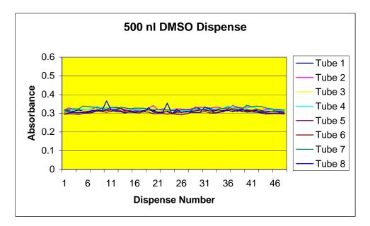
Figure 6. Valve-to-Valve Uniformity. DMSO containing a dye tracer (500 nl) was dispensed into a 384-well plate. After dispensing, 100 μl of water was added and the absorbance at 630 nm of each well was measured using a Synergy<sup>™</sup> HT Multi-Detection Reader. The data was then exported to Microsoft Excel and each valve tube's dispense was plotted separately.
