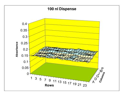
**Figure 5. Uniformity of Dispense.** The NanoQuot<sup>™</sup> Microplate Dispenser was used to dispense 100 nl of aqueous dye solution into 384-well microplates. After the addition of dye solution, 100 μl of diluent was added and the absorbance for each well determined. Data for the entire plate was plotted using Microsoft Excel.
