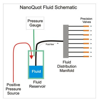
**Figure 2. Fluid Path Design of the NanoQuot.** Positive pressure drives fluids from the reservoir through a distribution manifold, which divides the fluid into 8 separate tubes. Eight precision valves control the fluid dispense into wells of the microplate. Pressure of the reservoir is monitored by a pressure gauge linked by tubing.
