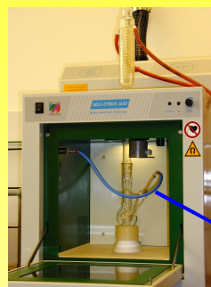
Milestone MLS 1600 Multimode Batch Reactor
