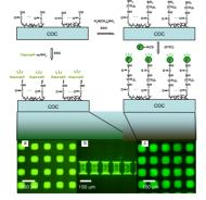
Eluorescent images of patterned poly(methacrylic acid) (a) on a COC sheet and (b)inside a channel of a COC microchip which labeled with Dapoxyl® dye. Image (c) was obtained by treated the pattern with ethylenediamine and then labeled it with a primary amine reactive dye, FITC.
