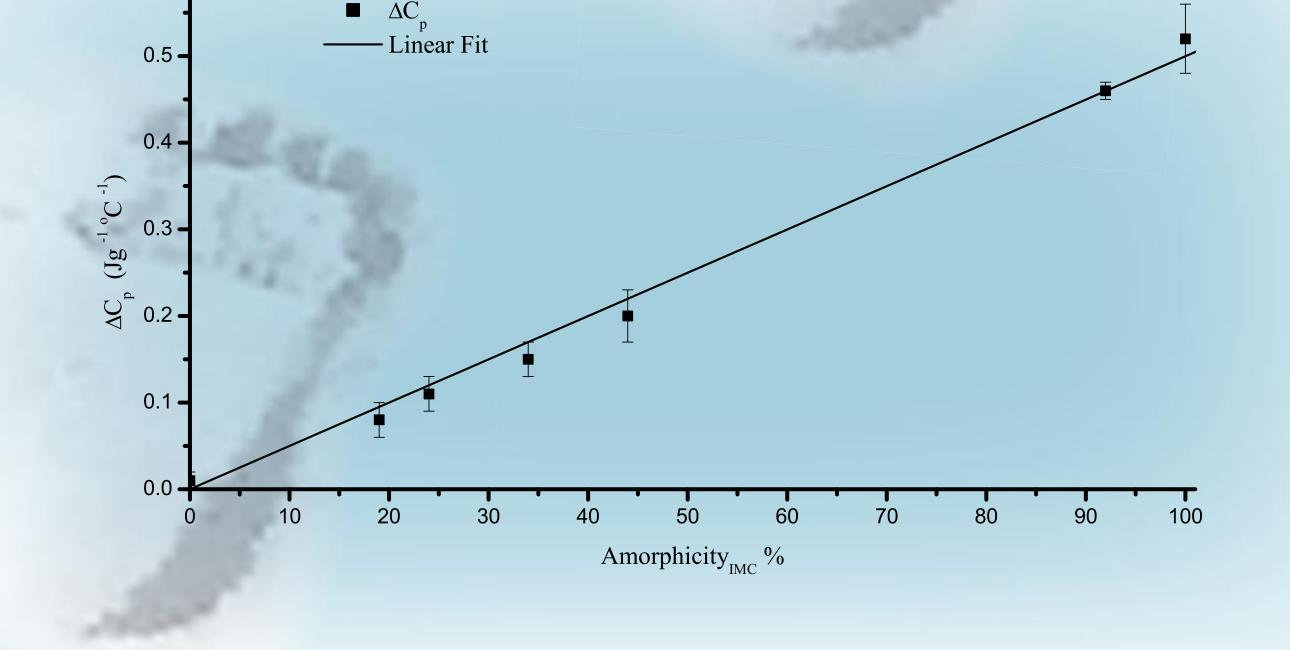
**Fig. 2.** StepScan DSC results for  $\Delta C_{p}$  at the glass transition are proportional to the amorphicity of lactose samples measured with IMC. The parameters of heating program are: Step size (2 °C), heating rate (5 °C/min), isothermal time (1 min) and equilibrium criteria (±0.01 mW).
