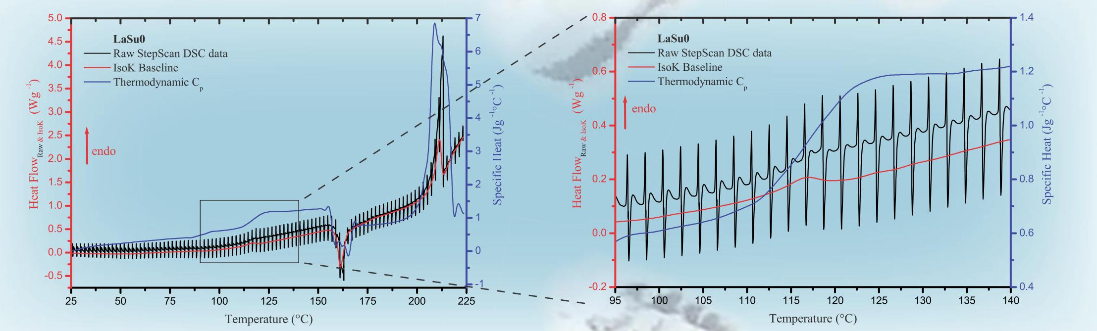
**Fig. 1.** From the raw StepScan DSC data can be calculated Thermodynamic  $C_p$  and IsoK Baseline curve. In this measurement the parameters of the heating program are: Step size (2 °C), heating rate (5 °C/min), isothermal time (1 min) and equilibrium criteria (±0.01 mW).
