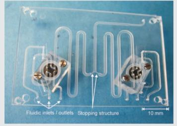
This picture shows a chip suitable for metering and merging two liquids by using two turning valves and a stopping structure. The chip is made of PMMA, structured by micromilling and covered with a polymer foil. The valves also consist of PMMA, bonded to an elastomer sheet working as a seal and containing two rotatable slots.
