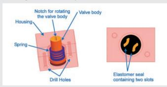
These CAD drawings show the build-up of the presented turning valve. A housing made of PMMA encloses a valve body (also made of PMMA), a metallic spring and an elastomer seal. The seal is glued to the valve body and contains slots. By revolving the valve body different fluidic channels can be connected. Depending on the designated purpose, slot shape and number can vary. In the drawing above, two fluidic channels are connected simultaneously.
