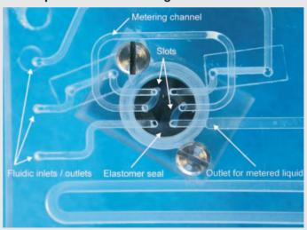
The picture above shows a closeup view of a metering structure. In this case the channels have a width of 0.6 mm. The metering channel together with the two slots possess a volume of 10 µl.
