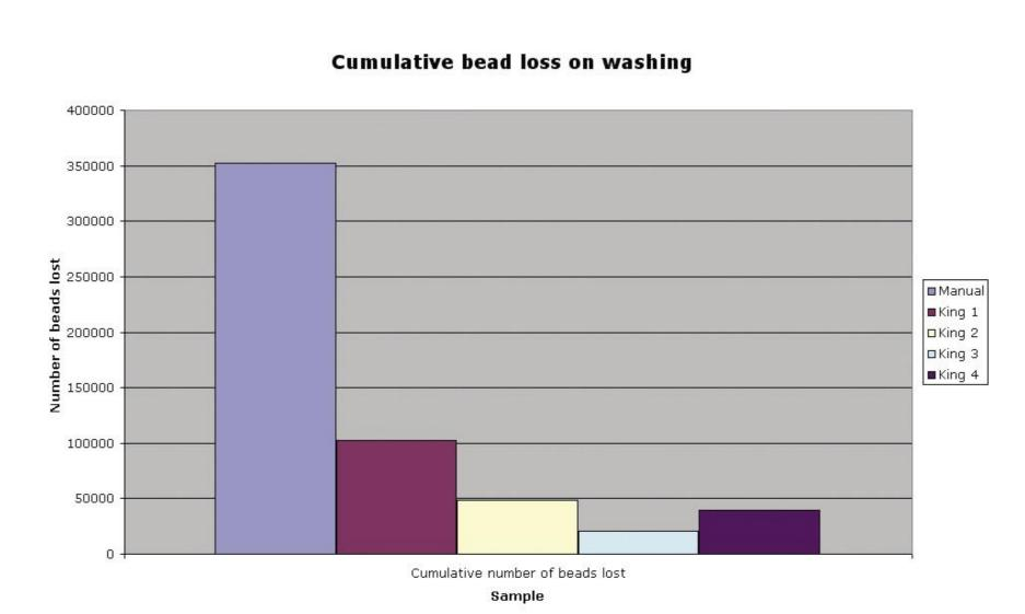
Figure 4. Comparison of the amount of beads lost during manual and KingFisher mL washings. During the KingFisher mL washings the collection of the beads is efficient and bead loss is minimal. Bead loss was shown as the cumulative loss over 7 washes.
