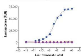
Variations of the ADCC Reporter Bioassay (FcγRIIIa-V158) were used to measure the Fc effector function of either Rituximab or Trastuzumab to demonstrate assay specificity. Similar results were obtained using all of the FcγR Reporter Bioassays referenced in panel 1 (data not shown).
