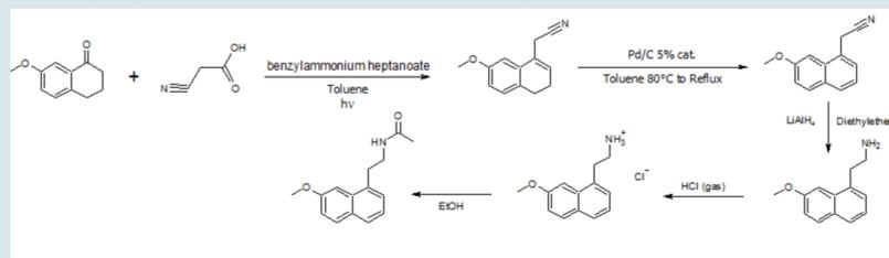
Figure 1—The process route for synthesis of Agomelatine.
