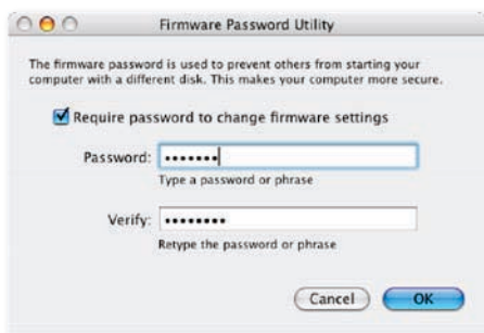
Figure 3: Administrators can use the Apple Firmware Password Utility to prevent unauthorized users from booting Mac workstations from external or optical devices or network resources.
