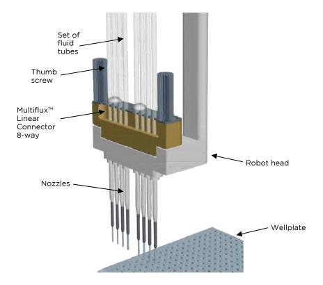
The Linear Connector 8-way engages directly with the robot head. By tightening down the two thumb screws a seal is made between the fluid tubes and the nozzles on the robot head. The perfluoroelastomer seal on the Linear Connector 8-way has very low dead volume and is chemically inert making it suitable for a number of different applications.
