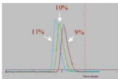
Overlay of 3 pairs of chromatograms obtained with 3 co-solvent contents
