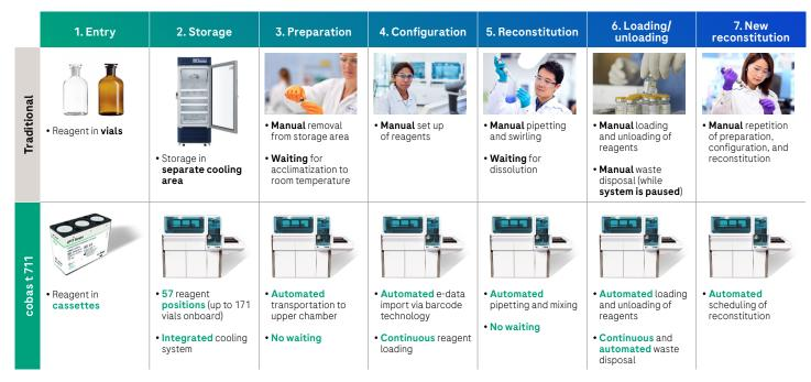
**Figure 2.** Traditional laboratory setting versus the walk-away reagent management (W.A.R.M.) concept with the **cobas** t 711 coagulation analyzer
